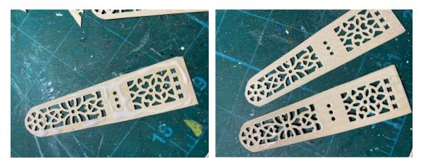
Ensure you interior pattern is lining up. If the outside edges aren't completely inline, no worries, we can sand the edges LATER. Here's an example of where the pattern is NOT lining up on the vane and one where it is lined up.
