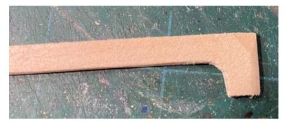
In addition to sanding the edge, cut a small sliver off the top edge for the riser to fit closely around the wooden disc on the underside of the tread.
