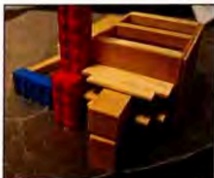
#4 Assembly of the shelf ends. Note the lego square checking to see if the ends are aligned.
