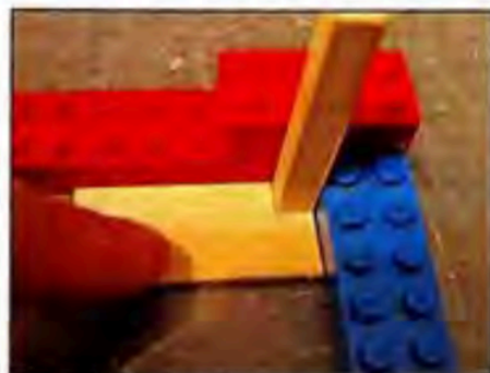
#1 Making the notched shelf with smaller 1/4" wide piece and 1/2" wide piece using the leg only as a spacer Do not glue to leg!
