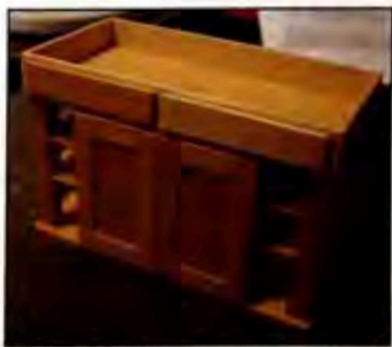
#6 Apron and bottom shelf glued to cabinet and legs.
