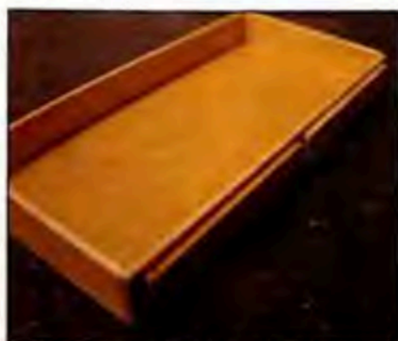
#2 Apron assembly. Note that the sides and front/back are glued around the apron support. Drawer fronts are glued on both sides of apron.
