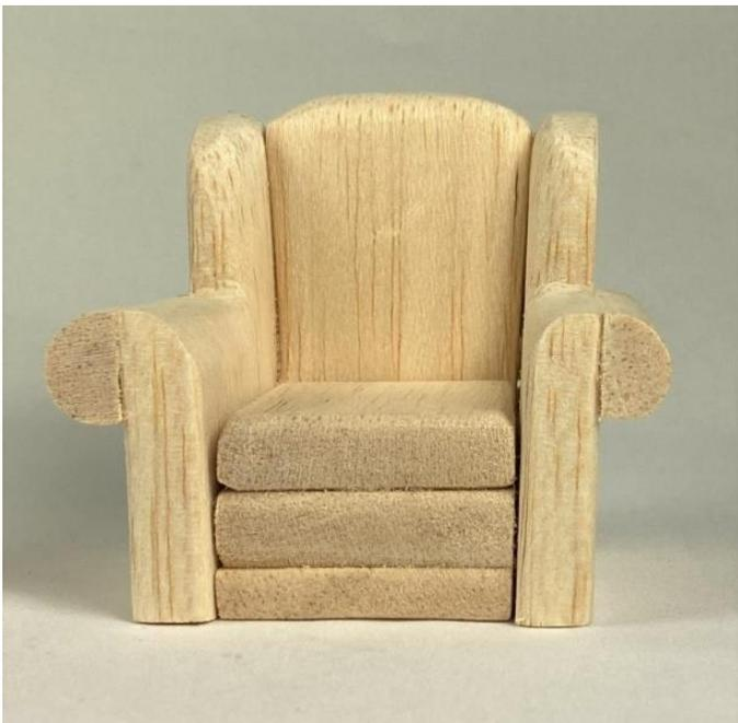
13. Cut 2 arms out of 3/8" thick balsa wood (you will start with two pieces about 9/16" wide and 2 1/8" long). Sand off the edges until you have roughly a half circle. Trial fit onto the sides, flush at the top of the arm, and glue into place.
