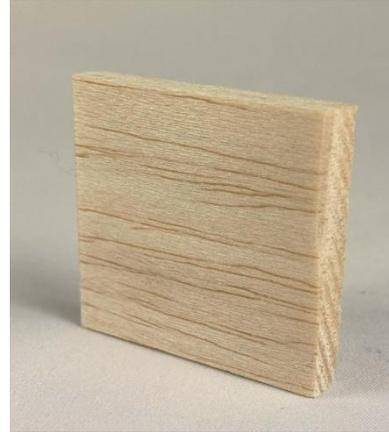
2. Slightly round off all the edges of one of the thick pieces for the top cushion by gently sanding off the harsh edges with an emery board.
