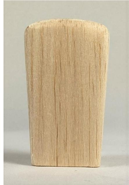
9. Cut 2 sides out of  $\frac{3}{8}$ " thick balsa wood (they will start out  $2\frac{5}{32}$ " wide x  $2\frac{5}{8}$ " high). Using your X-acto knife and a ruler, cut a taper on the back edge of the side to match the taper on the chair back. Rough cut the arm height and the curve of the wing using the illustration as a guide (you might even print the page and use it as a pattern). You will have one left side and one right side.
